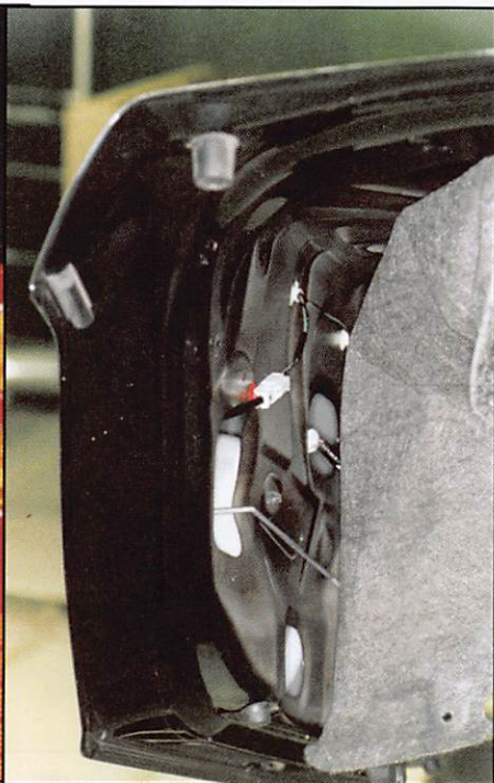
2. Next, we disconnect the lock rod.
